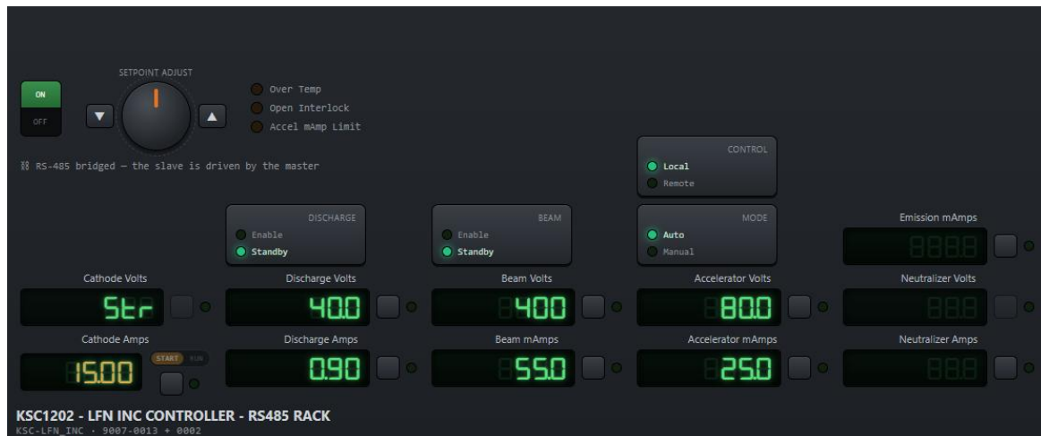
Figure 4. Kaufman source controller panel: Cathode, Discharge, Beam, Accelerator, Emission and Neutralizer with their Enable/Standby, Local/Remote and Auto/Manual selectors.
