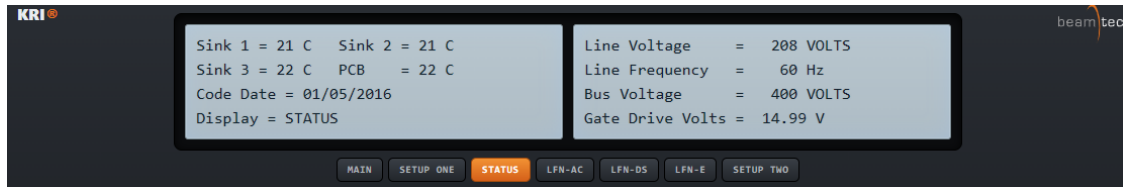
Figure 12. STATUS screen: sink/PCB temperatures, line and bus voltages, gate-drive voltage.
