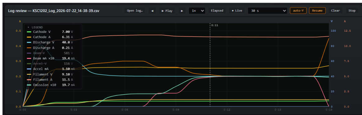
Figure 20. The same view with Beam V and Accel V switched off by clicking their legend entries (struck through). They drop out of the axis scaling — the left high-voltage axis disappears entirely and the remaining traces spread out over the freed height.
