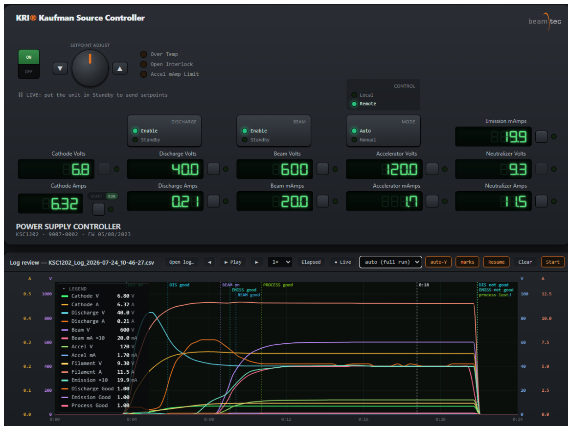
Figure 17. A real KSC1202 process under RS232 ACTIVE with marks on: the panel above; below, the discharge strike (cyan, settling to the 40 V setpoint), the beam ramp to 600 V / 20 mA at 20 mA emission, and the DIS / EMISS / BEAM / PROCESS “good” markers, with “not good” and “process lost” at switch-off.
