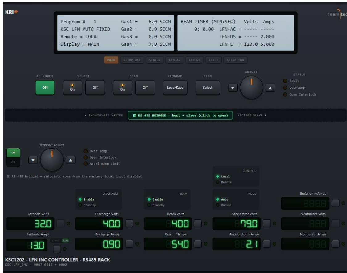
Figure 21. Replaying a recording onto a combined (RS-485 verbund) device: the cursor sample is written back onto the KSC1202 slave panel — note Beam Volts and Beam mAmps driven from the log.
