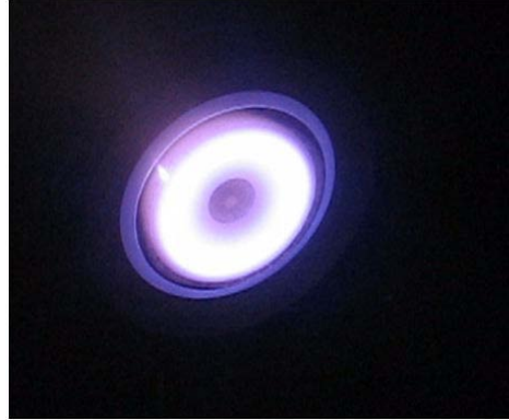
Same view & conditions as at left, but with plasma re-igniting - arcing is still decaying
