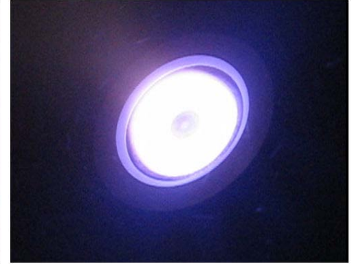
Arc suppression of Ion™ 1500 working in same environment & conditions - producing a stable plasma & good target utilization with negligible arc induced damage
